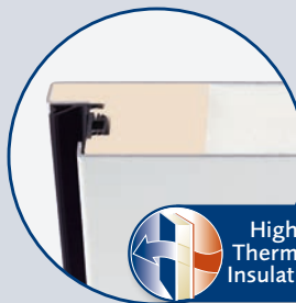
8 Thermal Insulation The door leaf is 46 mm thick and features a solid urethane foam core offering state-of-the art insulation to help you to reduce your energy cost.
