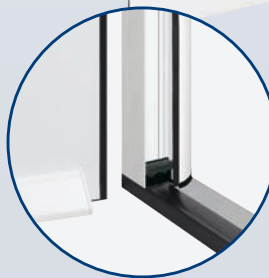
6 Aluminium/plastic threshold The door has a 20 mm high threshold with thermal break and a brush seal prevent heat from escaping near the floor.
